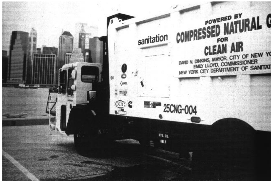
This sanitation truck in New York City powered by compressed natural gas as part of a Department of Energy managed trial and evaluation project.
