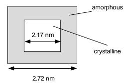
*Figure D.8.* Effects of confinement on the relative regions of the amorphous and crystalline areas.
